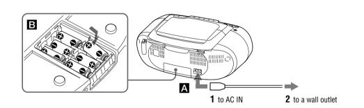
Connect the AC power cord A or insert six R14 (size C) batteries (not supplied) into the battery compartment B. Notes
